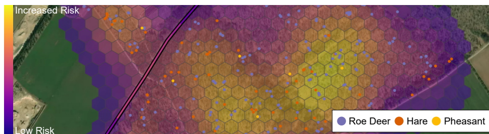
Fig. 1. Application of the risk model employing a GMM based on the precise positions of individual animals, as captured through drone recordings, and the nearby road.
